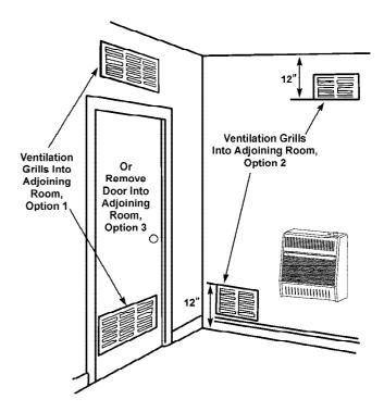
Figure 2-Ventilation Air from Inside Building
